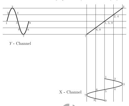
Divide the wave forms appearing an channel X and channel Y in equal parts, match the corresponding points on the screen. We would get a straight line in X - Y mode.
