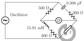
If the bridge is balanced for oscillator frequency  $f=2\,$  kHz, then the impedance Z will be
